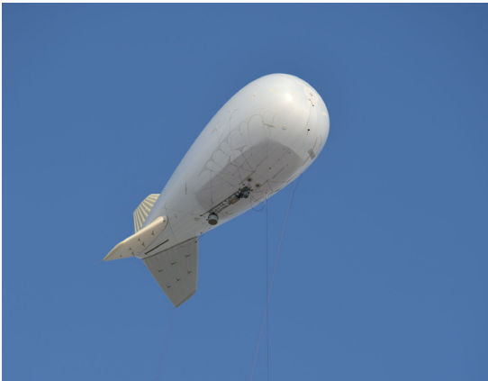
The aerostat used in the pilot project Maritime Surveillance Aerostat II
