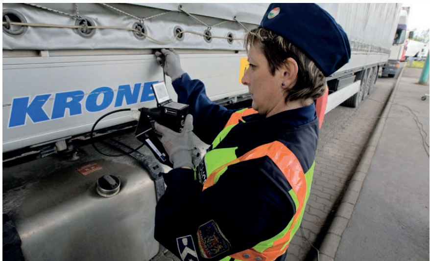
Figure 3. Hungarian police officer sets a sensor of a heart beat detector and a flexible camera to search for irregular migrants during control of a lorry at the border between Hungary and Serbia near Rösztke
